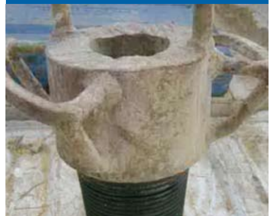
Homemade lift cap built from old drill collar pin.
