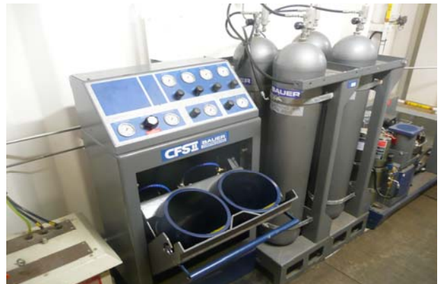
A dedicated self contained breathing apparatus refilling reduces the likelihood of contamination
