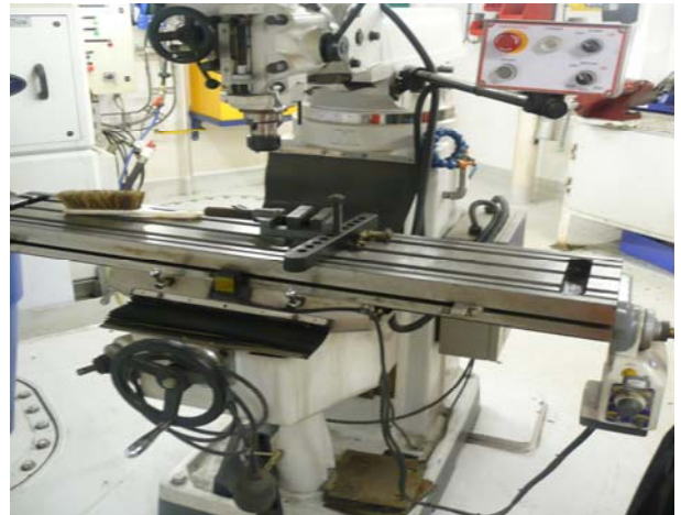
This workshop milling machine does not have guarding to protect its users from injury.
